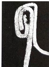
Roller 1: too narrow Roller 2: too loose
