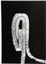
Roller 1: too loose Roller 2: normal
