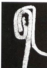
Roller 1: too narrow Roller 2: too loose
